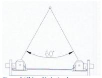
Figure 3 Lifting Chain Angles
