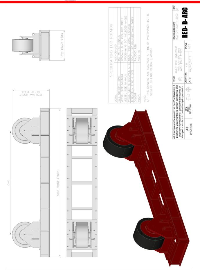
Figure 12 Idler Section GA Drawing & Specification
