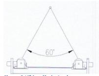
Figure 3 Lifting Chain Angles
