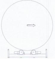
Figure 6 Wheel Brackets Too Close Together
