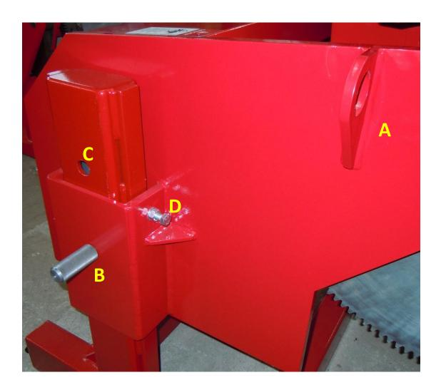
The table can then be raised or lowered by using the crane, so that hole C lines up with the lock pin (B) holes. Pin B on both sides of the machine can then be replaced. Once pins B are fully in place on both sides, then the weight of the table can be taken by the pins and the crane removed. Tighten the 4 bolts D (2 on either side of the machine), this will prevent any movement of the positioner inside the height adjustment sleeve.
