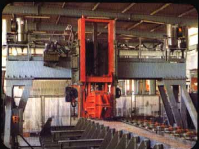
Twin Model 382 flux recovery systems, mounted on an overhead crane, return clean flux to two SAW flux hoppers on either side of the welding machine below.
