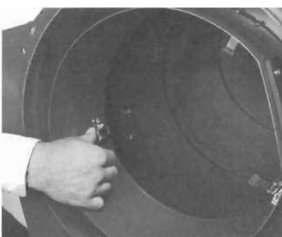
Reach up under tank and release (3) toggle clamps; make sure hooks are removed from bag ring.
