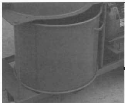
Release foot pedal; remove dust bucket.
