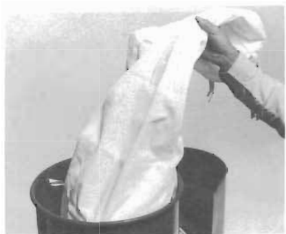
Pull bag up and shake to remove accumulated material.
