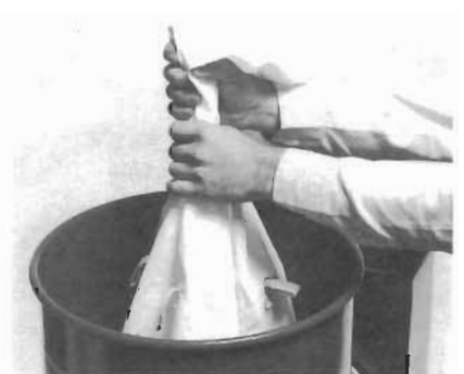
Grasp bag and lift bag ring out of tank.
