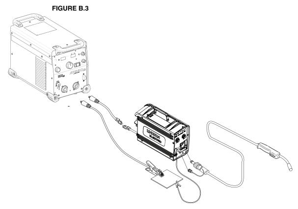
CrossLinc<sup>™</sup> - CrossLinc is a new welding system communication technology. When using a CrossLinc enabled power source such as the FX360XL and a CrossLinc enabled wire feeder such as the LN-25X, welding voltage can be controlled remotely without the use of an additional control cable.
