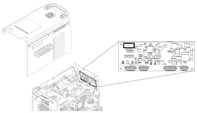
The User Interface pc board has one bank of dip switches. As shipped from the factory and under normal conditions, the dip switches are all in the 'off' position. There are 3 instances that require a change of the dip switch.
