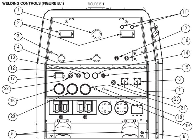
1. OUTPUT CONTROL- The OUTPUT dial is used to preset the output voltage or current as displayed on the digital meters for the five welding modes. When in the Arc Gouging or CV-WIRE modes and when a remote control is connected to the 3-Pin or 14-Pin Connector, the auto-sensing circuit automatically switches the OUTPUT CONTROL from control at the welder to the remote control.
