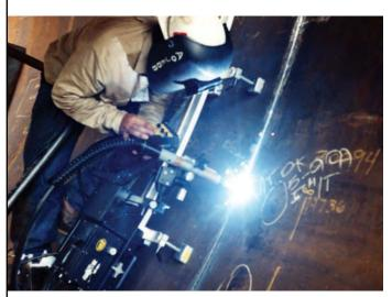
Shown Above - Vertical linear weave welding with ARM-2480 Support Bar w/ Magnets
