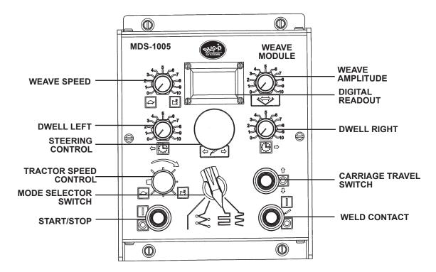
**AMPLITUDE (WEAVE):** Continuously adjustable up to a 2" (51 mm) maximum weaver stroke.
