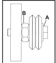
Check for proper alignment by using a finger to keep one of the wheels from rotating while manually moving the crossarm. The wheels are adjusted too tight if firm finger pressure is not enough to prevent wheel rotation. Once aligned, hold the adjustment bushing (B) still while tightening the hex bolt (A). Recheck alignment.
