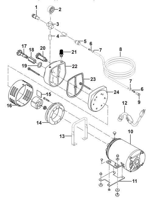
A Repair Kit ARV-1029 is available for the ARV-2020 and ARV-2030 pumps. The kit contains (4) vanes, (1) body gasket, filter felts for the muffler, oiler filter, and oiler wick, a cover gasket and separator felt for the oiler filter.
