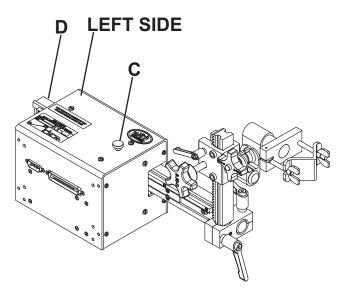
Set the weave amplitude to maximum. Use the steering knob on the control module to move the crossarm to both the extreme left and the extreme right. Perform measurements to determine if The crossarm is installed too far left or too far right. Repeat the crossarm realigning procedure changing the 1 7/8" (48 mm) dimension as required. Reinstall the two crossarm screws.
