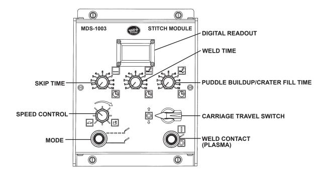
**SPEED CONTROL:** Sets the tractor weld speed from 2-120 in/min (5.1-304.8 cm/min).
