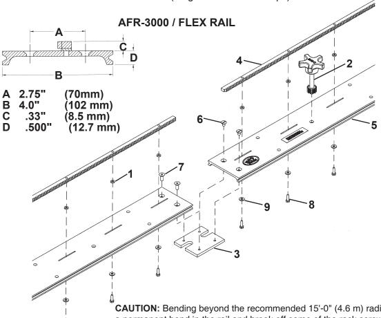
CAUTION: Bending beyond the recommended 15'-0" (4.6 m) radius may put a permanent bend in the rail and break off some of the rack screws.
